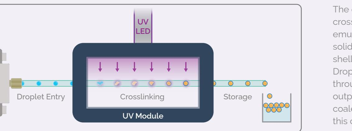
The optional UV module allows in-line crosslinking of droplets (single or double emulsion) of UV-sensitive material, so that solid beads and microcapsules with a solid shell and a liquid core can be easily produced. Droplets are isolated as they pass continuously through a glass capillary connected to the output of the Raydrop®, thus avoiding coalescence problems during this critical phase.
