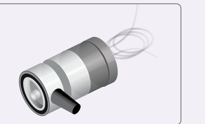
The Rheodyne™ sample injector allows a small volume of liquid to be loaded into a loop and then injected into the core or shell entry of the Raydrop®. During the injection step, the fluid from the loop is forced into the Raydrop® by the fluid coming from the core or shell phase reservoir.
