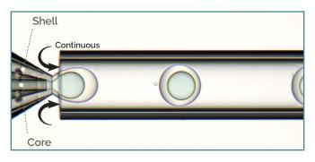
The way we produce droplets, particles and capsules relies on the use of couples of capillaries perfectly aligned in a metallic chamber. The first capillary is terminated with a 3D-printed nozzle and injects the droplet phase in the junction. The second one is the only output of the system, so it collects both phases, the droplet phase and the continuous phase filling the chamber under pressure.
